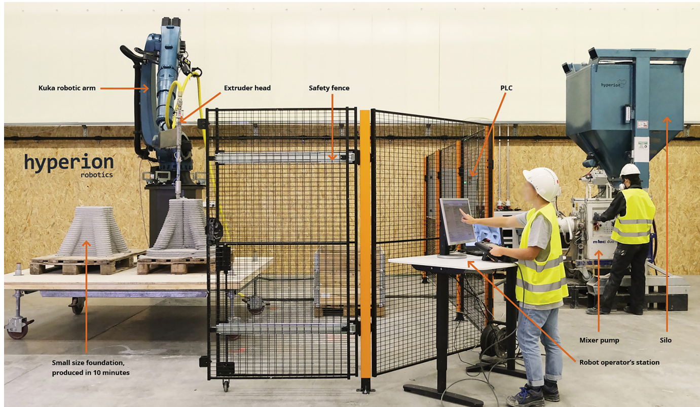
Figure 6.1 3D concrete printing facility in Espoo. (colour image is accessible via the link)
